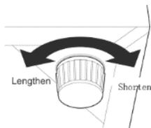
If the unit is not level, the doors and magnetic seal alignments will not be covered properly.
