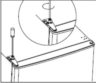
14. Click on the hinge cover and hole cover on the top of the unit.
