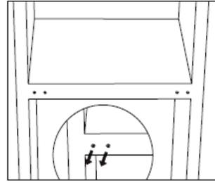
11. Stand up the unit and place the door on the bottom hinge. Make sure the bottom hinge core is inserted in the door hole. Then move the hinge hole cover of the bottom door from left to right side.
