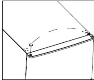
5. Unscrew the middle hinge and then lift the bottom door and put it on a soft pad to avoid scratches.
