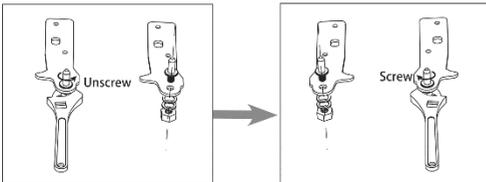
9. Install the hinge and foot base on the right side. Then fasten the two leveling feet back on.
