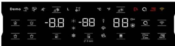
Press and hold Connect button for 3 seconds on Home screen. The Wi-Fi status indicator (⌚) on the refrigerator control panel will blink slowly while your refrigerator and router attempt to connect. If the connection is successful, the Wi-Fi status indicator will come on and remain lit.
